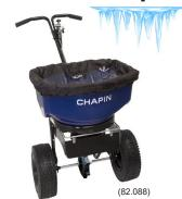
80-Pound capacity hopper with enclosed gear system to withstand the elements, supported by a rugged powder coated steel frame. Recommended for use with salt, halite/ice melt. Spiked auger tears up clumps. Adjustable front and side baffle system allows for precise control of spread pattern. Includes snow/rain cover and salt grate.
