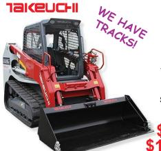
The Takeuchi TL8R2 tracked loader is a 9,200 lb. beast of a machine that has a 3000lb lift capacity at 50%. This is a High flow track loader. It has an impressive 6200lb bucket breakout force. Stop in and reserve our new skidsteer today!
